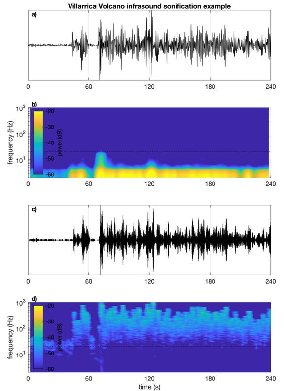
Figure 2: a) Infrasound collected at the Volcán Villarrica crater rim. b) Spectrogram calculated with 4 s windows and 2 s overlap. c) Processed infrasound using carrier frequency of 50 Hz and an index of modulation of 20. d) Corresponding spectrogram for panel c with 4 s windows and 2 s overlap. Spectrogram power is given in dB/Hz.
